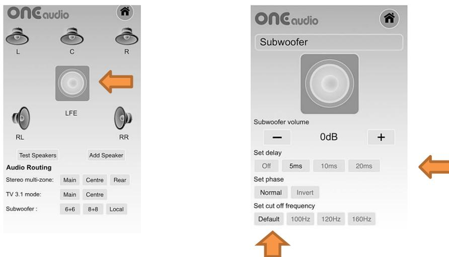
Set filter cut off frequency here, default is factory pre-set value which is tuned for the subwoofer
